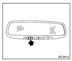
Using both hands, simultaneously push and hold both the HomeLink® button you want to program and the hand-held transmitter button.
