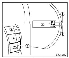
Odometer/twin trip odometer
