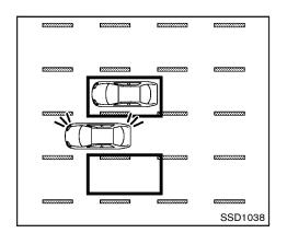
If the driver activates the turn signal, then the BSW indicator light flashes and a chime will sound twice.
