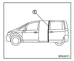
Be careful not to damage the sensor (1) of the sliding door.
