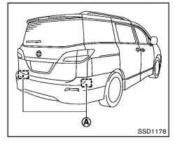
The BSW system uses radar sensors (A) installed near the rear bumper to detect other vehicles beside your vehicle in an adjacent lane.
