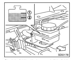
Check the fluid level in the reservoir. If the fluid is below the MIN line (2) or the brake warning light comes on, add Genuine NISSAN Super Heavy Duty Brake Fluid or equivalent DOT 3 fluid up to the MAX line (1). If fluid must be added frequently, the system should be checked by a NISSAN dealer.
