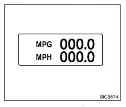
Average fuel consumption (MPG, I/100 km or km/l) and speed (MPH or km/h)
