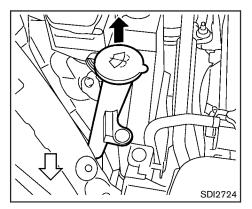
Fill the window washer fluid reservoir periodically. Add window washer fluid when the low washer fluid warning appears on the dot matrix liquid crystal display.
