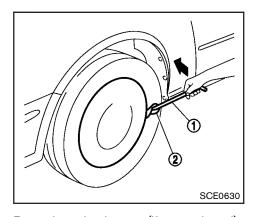
Removing wheel cover (if so equipped)
