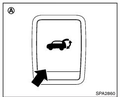
Power lift gate switch - Instrument panel
