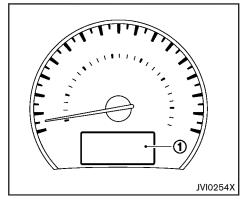
The dot matrix liquid crystal display ① is located in the speedometer, and it displays, the key operation information and other warnings and information.
