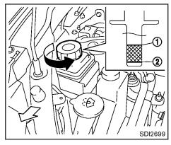
Check the fluid level in the reservoir.
