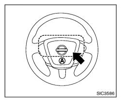
To sound the horn, push the pad area (A) of the steering wheel.
