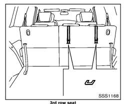
INSTALLING TOP TETHER STRAP (3rd row seat)
