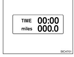
Elapsed time and trip odometer (miles or km)
